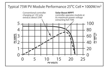
The actual charge current increase you will see varies primarily with module temperature and battery voltage. In comfortable temperatures, current increase typically varies between 10 to 25%, with 30% or more easily achieved with a discharged battery and cooler temperatures. What you can be sure of is that Solar Boost charge controllers will deliver the highest charge current possible for a given set of operating conditions.
