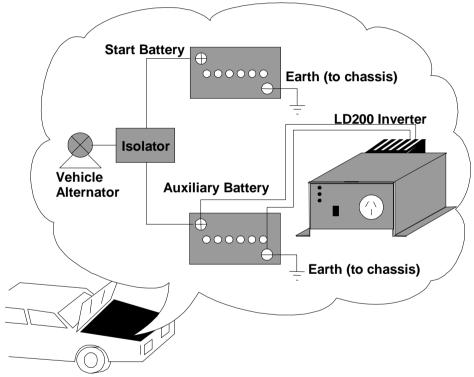
By incorporating an auxiliary battery in the manner above, the starting battery should remain charged for vehicle starting (see your auto electrician). The LD200 has sufficient battery cable length to allow it to sit underneath the vehicle whilst in use. If the ground is wet, place the LD200 on a waterproof liner.
