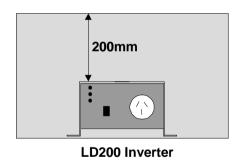
Please leave a clearance of 200mm on all sides and top of the Inverter. The LD200 must be installed in a dry, cool, dust-free environment. It is recommended that the inverter be placed as far from any radio receivers as possible.
