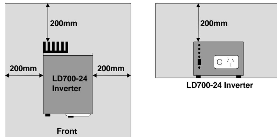
Please leave a clearance of 200mm on all sides and top of the Inverter. The LD700-24 must be installed in a dry, cool, dust-free environment. It is recommended that the inverter be placed as far from any radio receivers as possible.
