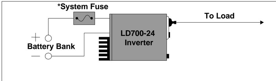
\* A system fuse (of at least 35 Amps) should be placed before the battery. An HRC motor start type is recommended. (See your system designer for details).
