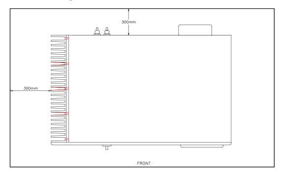
We suggest that you house your Inverter and other power generating equipment in a purpose built shed remotely sited from the home, and as far away as possible from any radio transmitters or receivers. Also make sure that the exhaust from your generator or other sources of heat or fumes are kept well away from the SE22. SEIAA (Solar Energy Industries Association of Australia) installation guidelines must be followed.
