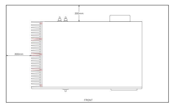
We suggest that you house your Inverter and other power generating equipment in a purpose built shed remotely sited from the home, and as far away as possible from any radio transmitters or receivers. Also make sure that the exhaust from your generator or other sources of heat or fumes are kept well away from the SE32. SEIAA (Solar Energy Industries Association Of Australia) installation guidelines must be followed.
